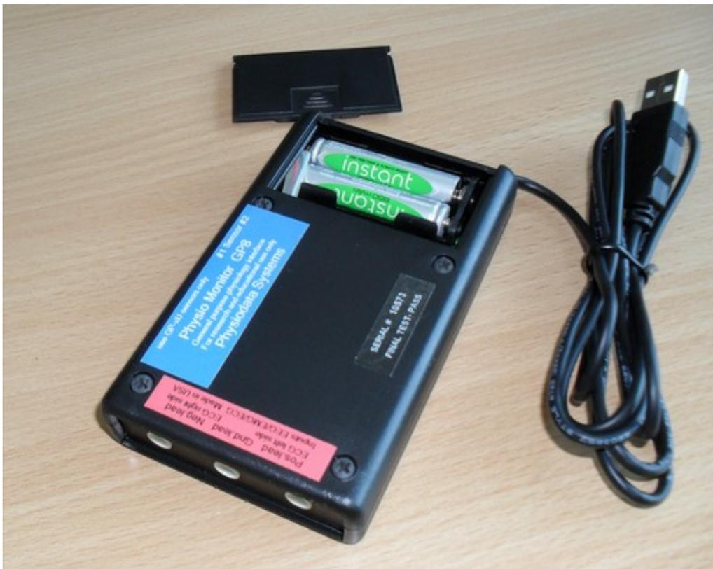
Figure 2 – GP8 amplifier underside with battery cover removed
