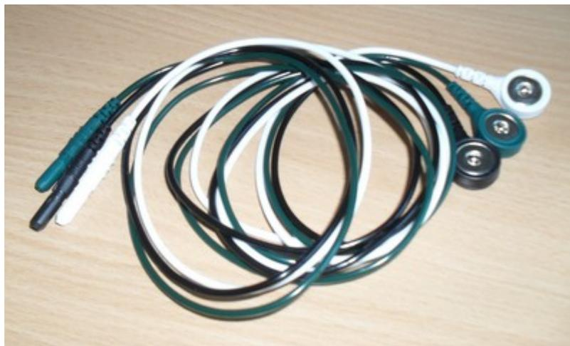
Figure 3 – Set of 3 cables (TP40) used for EMG and EKG. The plugs at the left side are inserted into the GP8 unit. The heads (right side) need to be fitted with snap electrodes (e.g. see figures 4,5 and 6) before being attached to the skin.
