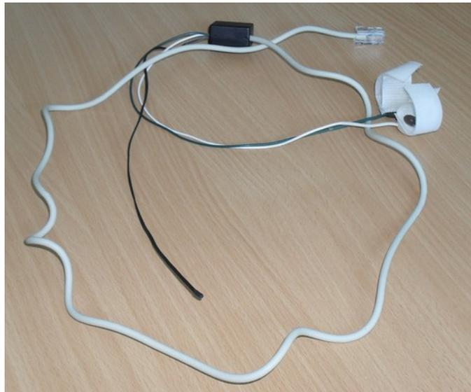
Figure 7 – Temperature sensor (black cable) and skin conductance sensors (white velcro straps)
