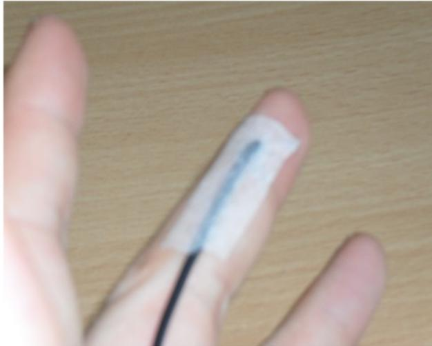
Figure 9: Skin temperature sensor placement
