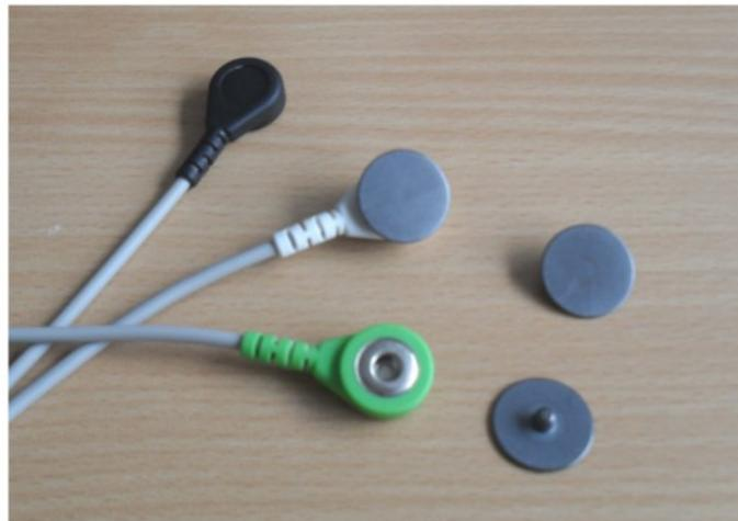
Figure 5 – Gel-free reusable snap electrodes for use with cable MC-5SGW
