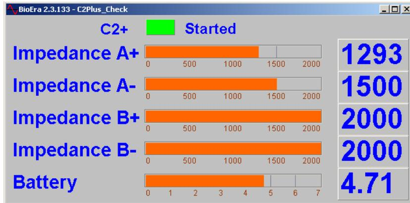
Figure 10: Battery and impedance checking application
