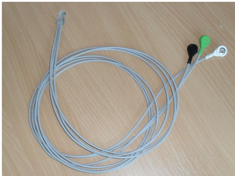
Figure 3 – Set of three cables for EMG. The heads (upper right) need to be fitted with snaps (see figures 5 and 6).
